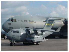
The base of the C-17 replica is a John Deere "Gator" multi-purpose vehicle, donated by the 315th Recruiting Service. The replica is 32 feet long, 13.4 feet tall, has a wingspan of 28.5 feet and was built in modules to make
